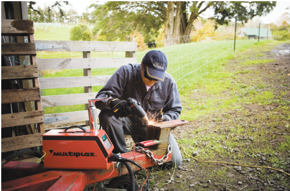
Not much bigger than an old-time radio, all the Multiplaz 3500 welder needs is 110 or 220-volt current, water and alcohol.
