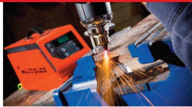
FIGURE 2 The equipment's plasma flame can cut up to 0.375-in.-thick plate and still deliver a clean cut.
