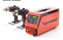
Multiplaz employs unique welding technology by use of a water-alcohol solution instead of shielding gas. The Multiplaz 3500 can weld, solder, braze, harden, and cleanse metals including steel, aluminum, copper, cast iron, bronze and other metals. The machine can cut any metal, including high-alloy and stainless steel that cannot be cut with oxygen cutting as well as cut ceramic tiles, quartz glass, bricks, concrete and other inflammable materials. www.multiplaz.com
