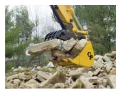
Available in 10- to 84-in. widths with various teeth styles, CP Heavy- and Severe-Duty Buckets aggressively handle the most abrasive materials with excavators up to 200,000 lbs. A circular torque tube design enhances strength. One-piece T-1 curved side cutters, side wear pads, and an abrasion-resistant double bottom protect against premature wear. Heavyduty bucket capacity sizes range from 0.037 to 5.7 cu yds; severe-duty from 0.106 to 3.9.
