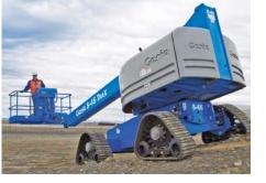
height of 40 ft and a vertical reach of 31 ft, and the S-45 Trax has a lift height of 46 ft and a vertical reach of 36 ft. The booms offer traditional front-wheel steering with a 30-degree steer angle. **www.terex.com**
