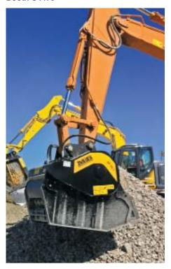
Attach the Crusher Bucket to an excavator to crush reinforced concrete and other material right in the bucket, eliminating the need to haul waste to a dump by returning clean rebar and material that's ready to be reused. Four models fit excavators 9 tons and larger. www.mbamerica.com/eng
