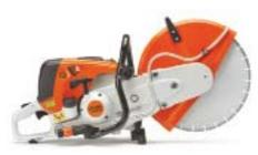
TS 410 A (EWC) Cutquik Cutoff Machines offer control over water flow to the cutting surface. The EWC stops the water flow at idle speeds and automatically starts again when the throttle is fully engaged. Offers an anti-vibration system, mounted keypad, and an X2 low-maintenance air filter system.
