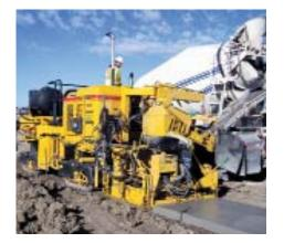
The GT-3200 sidewalk paver can be equipped with a front-mounted adjustable aggregate base mold to spread base aggregate for a sidewalk. The paver has a 20-in.-wide, 14-ft-long folding conveyor. The conveyor allows ready-mix trucks to discharge from the street instead of driving over curbs to reach the paver. The paver also features all-track steering. www.gomaco.com
