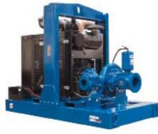
With discharge sizes up to 8 in., Prime Aire Plus pumps offer increased head flow. They fit many other pumping installations and support clear liquids or liquids with solids. Features include 4950-gpm maximum flow and heads to 475 ft. They're available coupled to EPA-compliant engines or electric motors. www.grpumps.com
